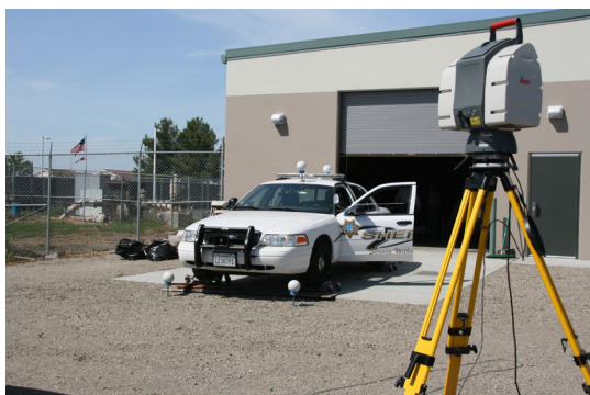
Leica ScanStation II measuring Patrol Vehicle with Ballistic Trajectory Rods inserted into bullet holes
